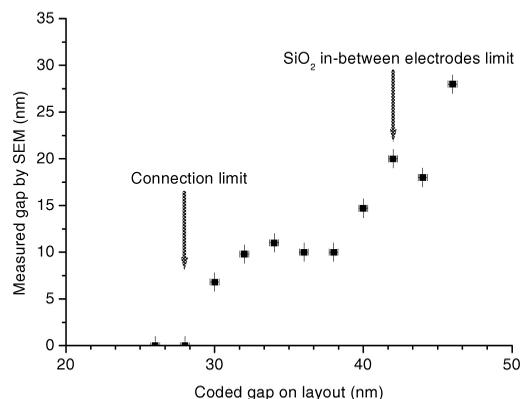
Fig. 3. Experimental evolution of the inter-electrode gap size as a function of the spacing coded in the layout of the pattern.
