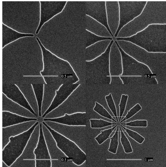
Fig. 4. SEM image of three, six, eight and ten nano-electrodes patterns after etching of the silicon substrate.
