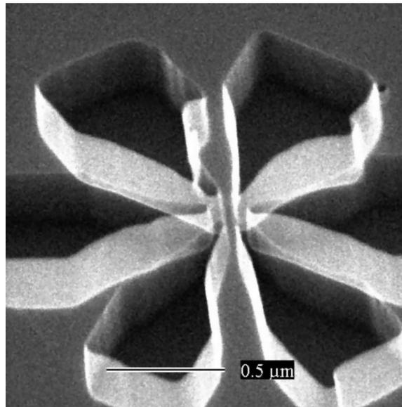
Fig. 6. SEM tilted image of a six nano-electrodes mold pattern after HREBL and 300 nm depth etching of silicon and O<sub>2</sub> plasma cleaning.
