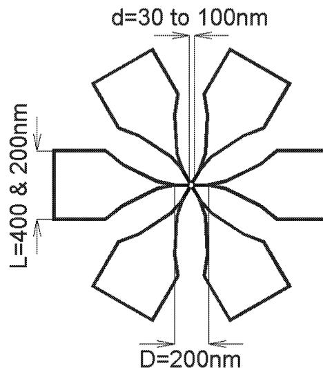
Fig. 1. Example of layout of a pattern comprising six nano-electrodes.
