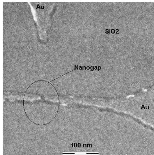
Fig. 2. SEM image of two embedded gold nano-electrodes separated by 7 nm used for carbon nanotubes connection. Lateral gate electrodes have been added for electronic transport modulation.
