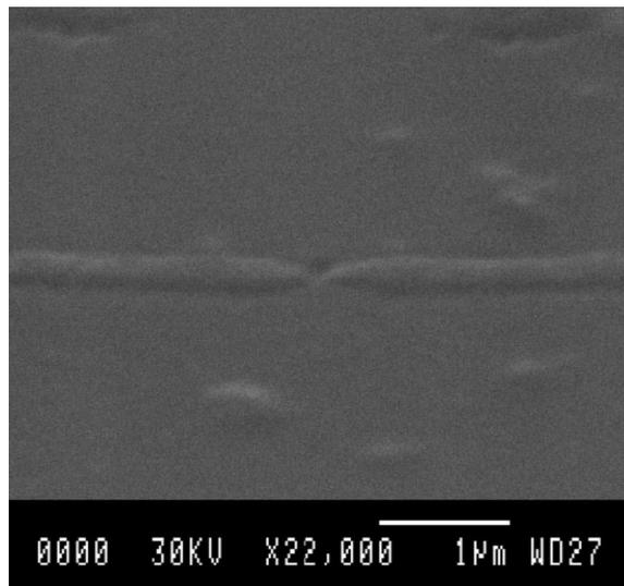
Fig. 7. SEM image of a pattern of two nano-electrodes (200 nm wide, separated by a gap of 50 nm) imprinted in PDMS using a negative master.
