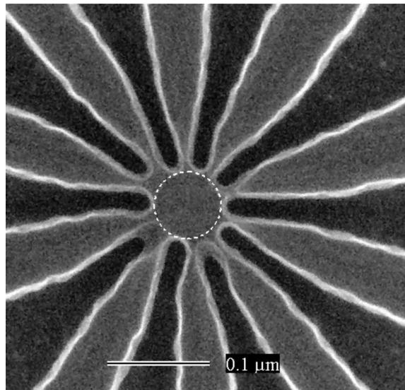
Fig. 5. Enlarged SEM image of the ten nano-electrodes pattern exhibiting an inter-electrode area diameter of 65 nm (dotted circle).
