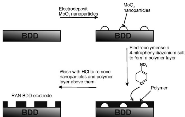
Scheme 2. A cartoon showing the three-step process to fabricate the RAN BDD electrode.
