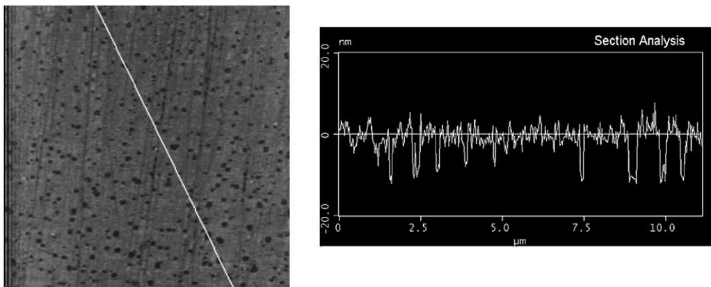
Fig. 3. The 2D AFM image of the RAN BDD electrode surface showing the corresponding line segment analysis across several BDD nano-discs.
