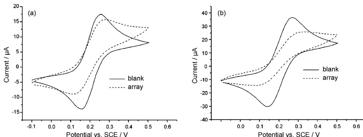
Fig. 4. The cyclic voltammetric response of both a bare BDD and a RAN BDD array in a 1.0 mM solution of potassium ferrocyanide at (a)  $200 \text{ mV s}^{-1}$  and (b)  $1000 \text{ mV s}^{-1}$  showing the switch between the different types of diffusional behavior (see text).
