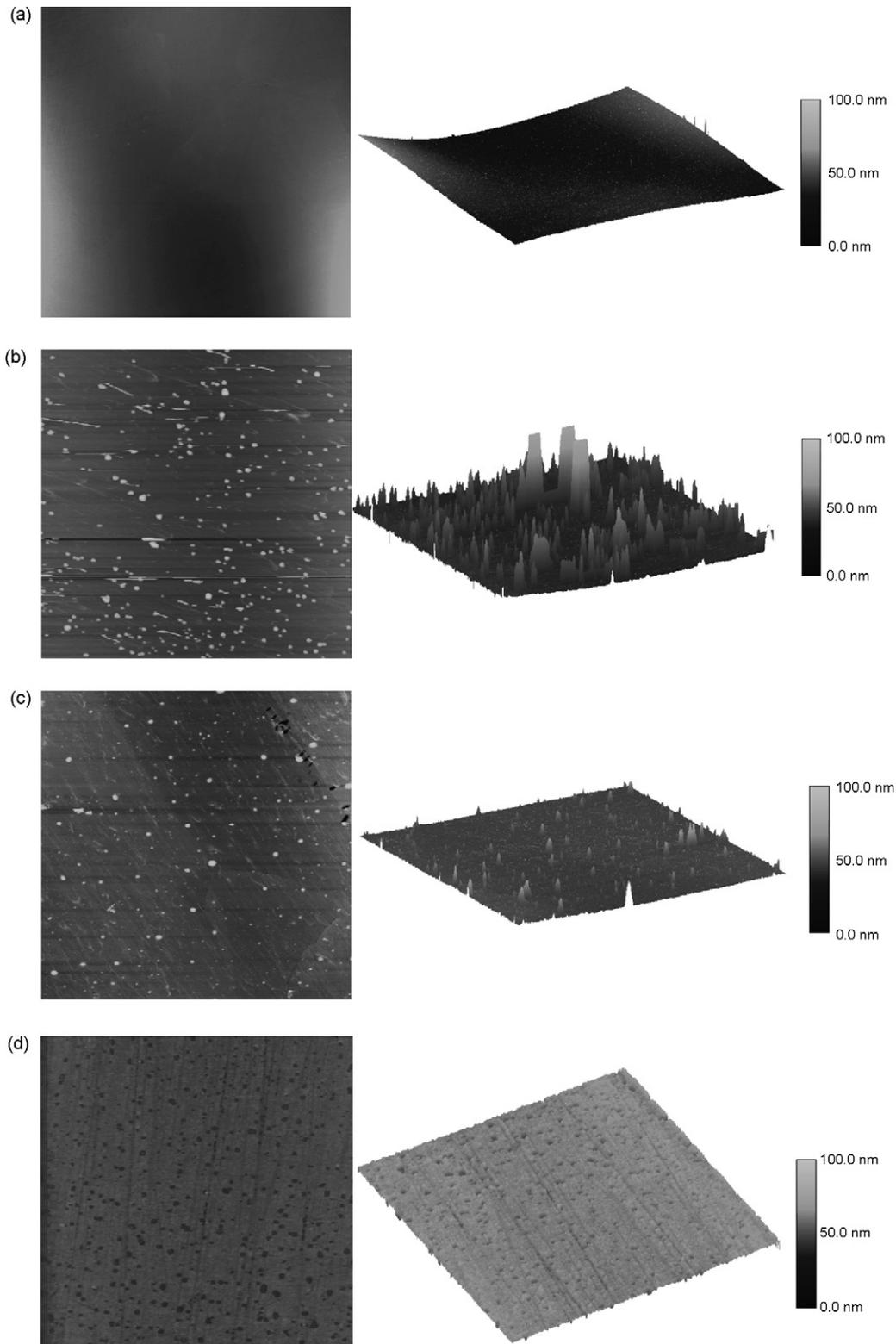
Fig. 2. AFM images showing the 2D (left) and 3D (right) surfaces of: (a) the bare BDD electrode; (b) the MoO<sub>2</sub> nanoparticle modified electrode; (c) the polymer film covered electrode; (d) the RAN BDD electrode.
