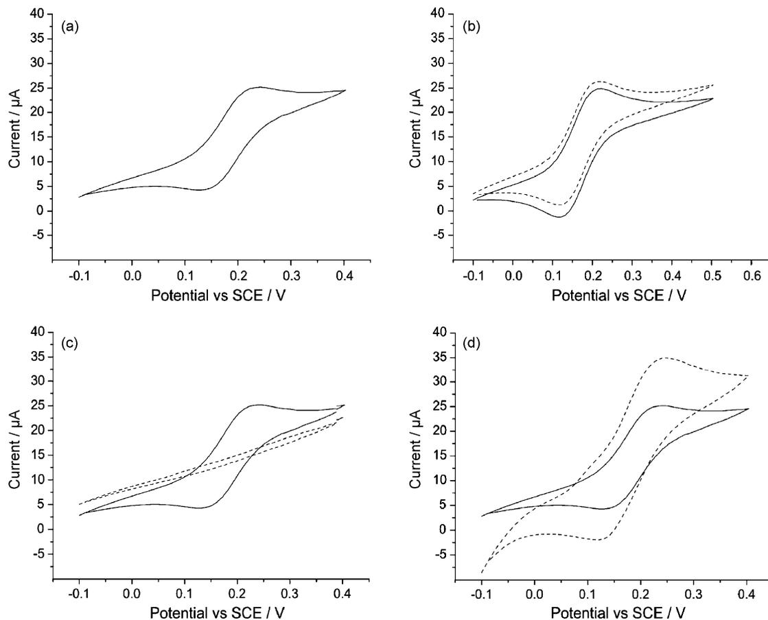
Fig. 1. The cyclic voltammetric response (scan rate  $100$  mV s<sup>-1</sup>) of a 1.0 mM solution of potassium ferrocyanide at: (a) the bare BDD electrode, (b) the MoO<sub>2</sub> nanoparticle modified BDD electrode (solid line) compared to the response at the bare BDD electrode (dashed line); (c) the polymer film covered electrode (dashed line) compared to the bare BDD electrode (solid line); (d) the RAN BDD electrode (dashed line) compared to the bare BDD electrode (solid line).
