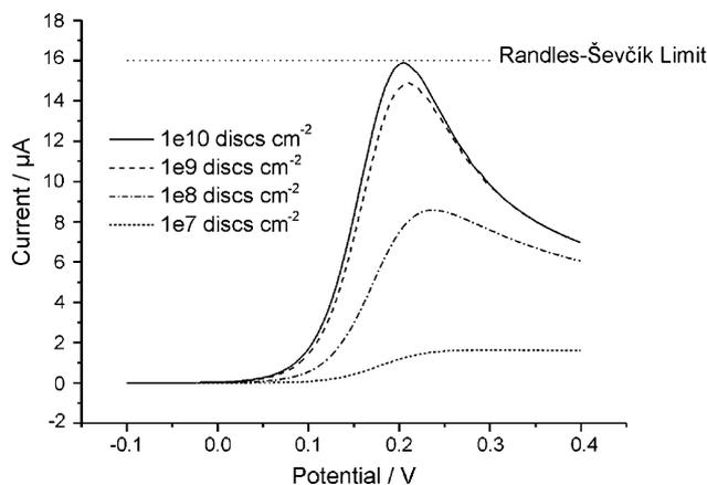
Fig. 5. Numerically simulated voltammograms for a regular array of nano-disc electrodes (radius = 10 nm) with varying numbers of electrode discs per unit area at a scan rate of  $100 \text{ mV s}^{-1}$  in  $1.0 \text{ mM}$  potassium ferrocyanide.
